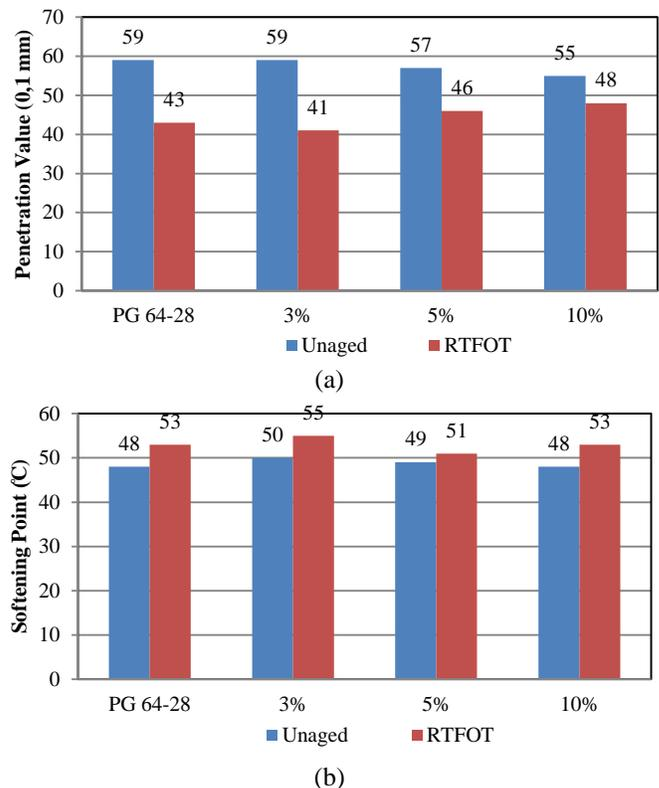
Fig. 2. Empirical Properties of Neat and Modified Binders, Unaged and RTFOT Aged: (a). Penetration; (b). Softening Point
