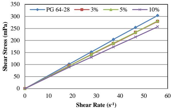
Fig. 3. Flow Curves of Original and Modified Binder at 135°C
