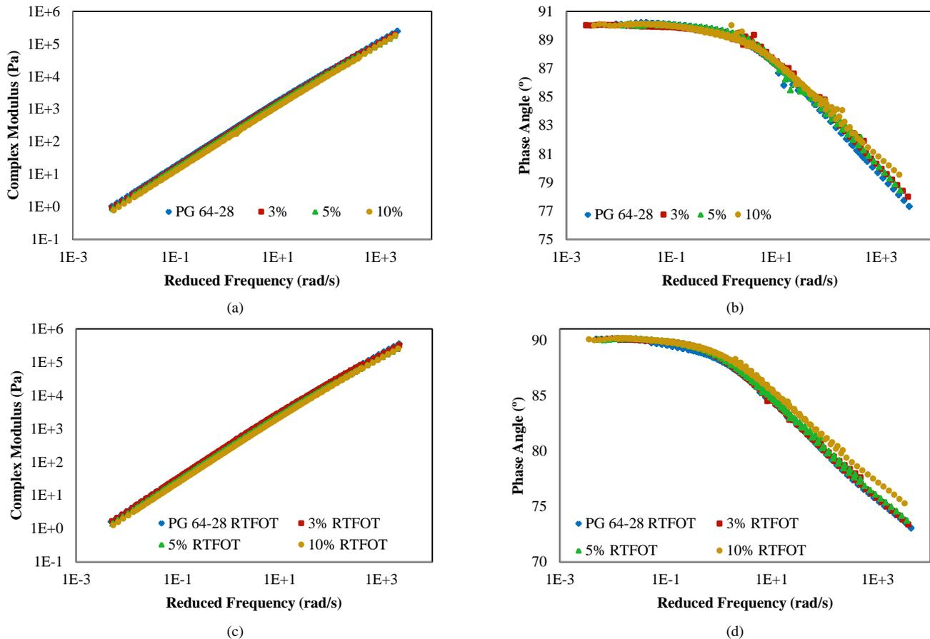
Fig. 5. Master Curves as Function of Frequency at 65°C: (a)  $G^*$  and (b) Phase Angle for Unaged Samples; (c)  $G^*$  and (d) Phase Angle for RTFOT Aged Samples
