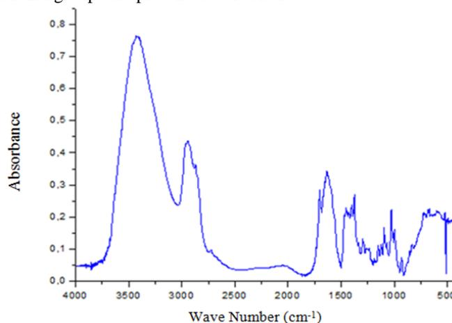
Fig. 1. FTIR spectrum of the sap, from 4000 $\text{cm}^{-1}$  to 400  $\text{cm}^{-1}$  wave numbers
